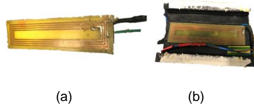
Figure 6. a) Inductor moving coil; b) Steady receiver coil.
