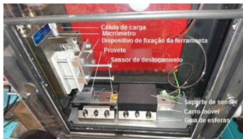
Figure 3. Test machine developed by Fernandes (2017) for high speed metal cutting tests.
